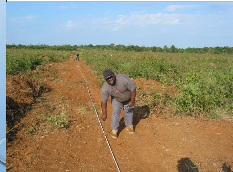
Photo of an array deployed in Puerto Rico to investigate sinkholes.
